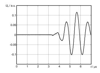
Fig. 2. The 1.0 MHz frequency signal passed through 2.5 mm thickness of PE80 type polyethylene test sample used as the reference signal for estimation of ultrasound velocity by crosscorrelation technique
