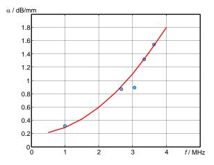
Fig. 10.The dependency of attenuation of ultrasound longitudinal waves propagated in the PE80 type polyethylene on frequency
