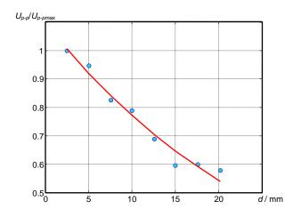
Fig. 7. The normalized peak to peak amplitudes of the signals received at different distances at the frequency 1.0 MHz and the approximated curve of ultrasound attenuation
