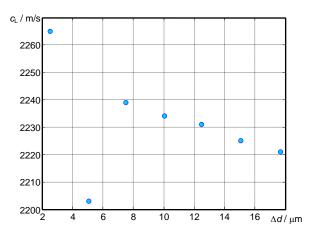
Fig. 3. Measured velocities of longitudinal waves obtained for different propagation distances at the frequency 1.0 MHz
