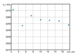
Fig. 5. Measured velocities of longitudinal waves obtained for different propagation distances at the frequency 5.0 MHz
