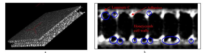
Fig. 10. a - CT specimen, b - frontal section CT specimen with porosity areas
