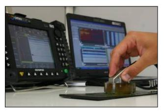
Fig. 3. Phased Array semi-automatic system
