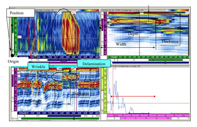
Fig. 13. UT phased array representation
