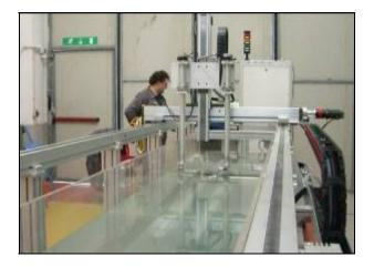
Fig. 1. BYTEST immersion ultrasonic system
