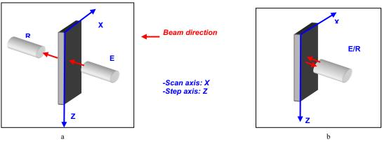
Fig. 12. a – pulse-echo technique, b - through transmission technique
