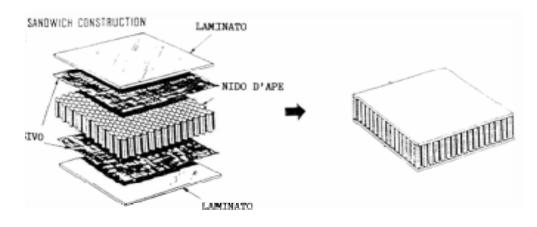
Fig. 9. Honeycomb structure
