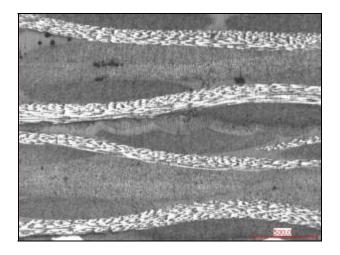
Fig. 6. Micrographic evidence to 50X cross-section of a sample with evidence of both elongated and isolated porosity areas
