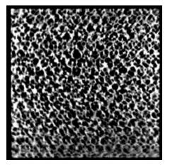
Fig.16. CT section sandwich structure
