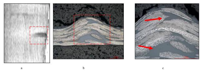
Fig. 11. a – c-scan representation in amplitude, b – micrographic evidence to the wrinkle 25X, c - detail of the same at 50X (See dashed area in the previous photo). The arrows indicate areas with the highest concentration of resin.
