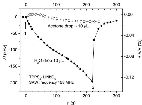
Fig. 4. SAW oscillator frequency change  $\Delta f$  and the correspondent relative change  $\Delta V/V$  in SAW velocity as a function of time: (1) piece of wet paper inserted and the cavity closed; (2) cavity opened and paper removed. Open circles show the oscillator response to acetone vapour.
