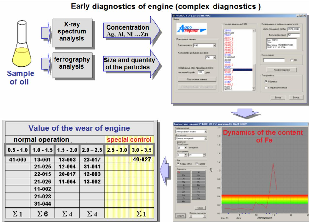
Fig. 1. The structural scheme of the organization of the work (researches) in the tribomonitoring field
