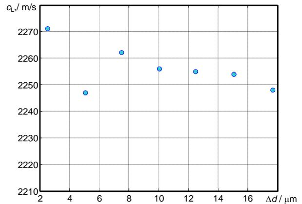
Fig. 5. Measured velocities of longitudinal waves obtained for different propagation distances at the frequency 5.0 MHz
