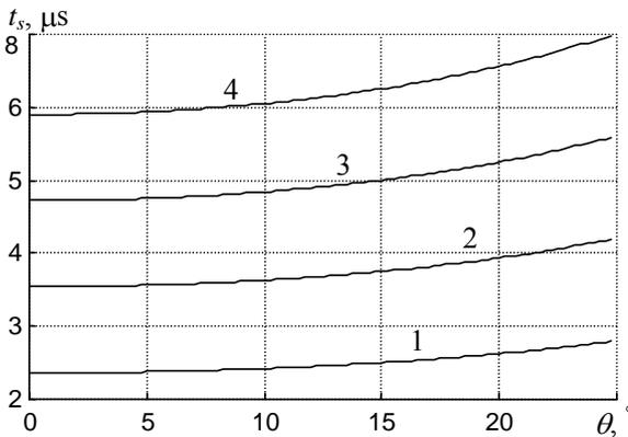
Fig.3. The dependence of time propagation  $t_s$  of shear waves in the glass pane on the angle of incidence  $\theta$  ( $\theta$  is less than the first critical angle), when the thickness of glass pane  $h$  is changed: 1- $h=4$ mm, 2- $6$ mm, 3- $8$ mm, 4- $10$ mm
