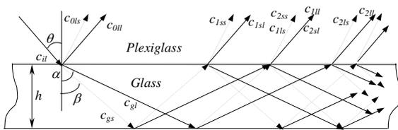
Fig.1. The propagation of ultrasound waves in a glass pane
