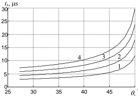
Fig.5. The dependence of propagation the time  $t_s$  of shear waves in the glass pane on the angle of incidence  $\theta$  ( $\theta$  is between the first and second critical angles), when the thickness of glass pane  $h$  is changed: 1- $h=4$ mm, 2- $6$ mm, 3- $8$ mm, 4- $10$ mm
