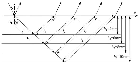
Fig.6. Schematic diagram of the measurement of thickness of glass panes by the shear waves
