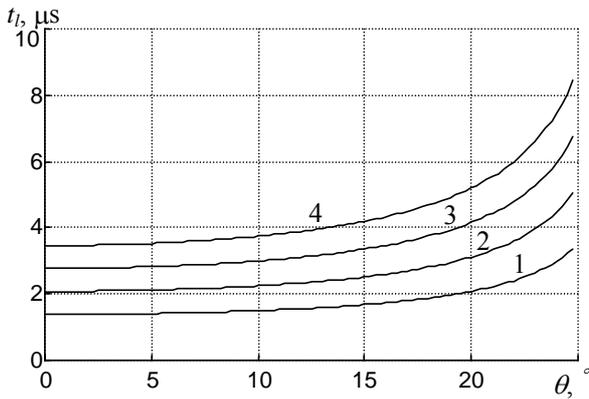
Fig.2. The dependence of time propagation  $t_l$  of longitudinal waves in the glass pane on the angle of incidence  $\theta$ , when the thickness of glass pane  $h$  is changed: 1- $h=4$ mm, 2- $6$ mm, 3- $8$ mm, 4- $10$ mm.
