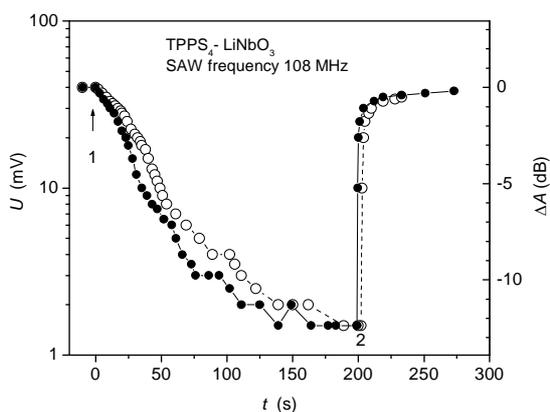
Fig.3. SAW pulse amplitude  $U$  at the output transducer and the correspondent change in SAW attenuation  $\Delta A$  as a function of time: (1) piece of wet paper inserted and the cavity closed; (2) cavity opened and paper removed. Two consequent experiments with the time interval of 300 s are represented by full and open circles.
