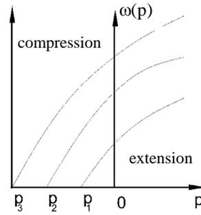
Fig. 3. Dependence of eigen frequencies of the transversal of the shell on the compression and extension
