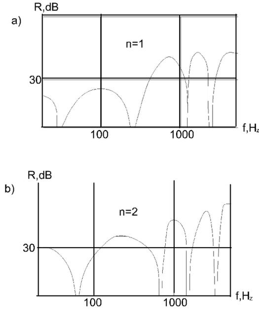
Figs 4. Sound insulation of the cylindrical shell ( $h=2$  mm,  $R_r=300$  mm) in air at the multipole ( $n=1$  and  $n=2$ ) sources of sound, located on the axis
