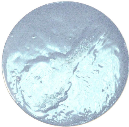
Fig. 3. Visible light image of a metallic plate surface under paint. Diameter of the plate is 76 mm.
