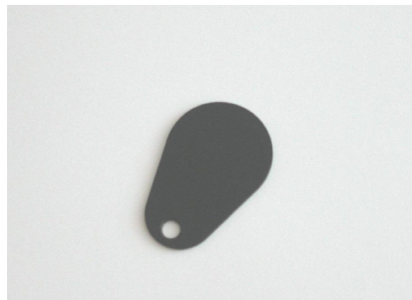
Fig. 2. Visible light image of a door electronic key transponder.
