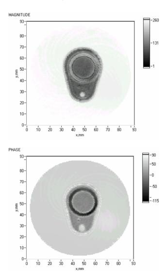
Fig. 4. Millimetre wave amplitude (top) and phase (bottom) images of the door electronic key transponder. Wave frequency is 120GHz.
