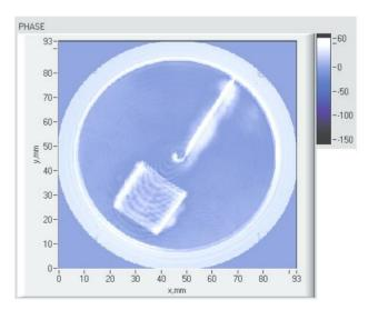
Fig. 5. Millimetre wave amplitude (top) and phase (bottom) images of the metallic plate with local destructive surface under paint. Wave frequency is 120 GHz.
