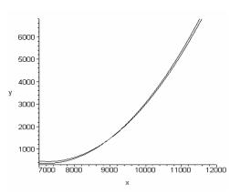
Fig. 1. Characteristics of draft of the engine (y) depending on frequency of rotation KVD, SNE and PPR (x) (SNE - from the beginning of operation, PPR - after last repair)
