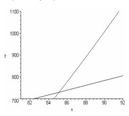
Fig. 2..2. Dependence of the temperature of gases behind the turbine of the engine of the aircraft (y) on frequency of the second cascade when there was a malfunction (x)
