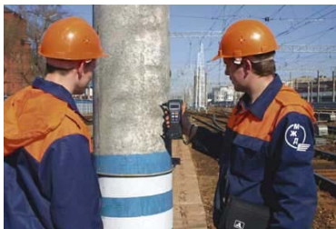
Fig. 11. UT tester UK1401. Testing of contact line support
