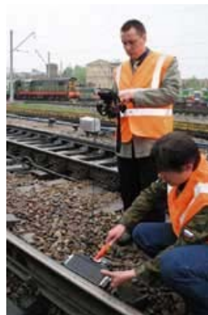
Fig. 14. Rails testing process with the guided wave flaw detector AKR 1224
