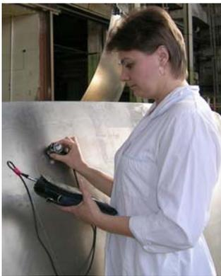
Fig.16. Process of thickness measurement
