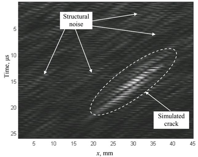
Fig.1. Simulated *B-scan* image of the intergranular stress corrosion crack, which is covered by the background of the structural noise
