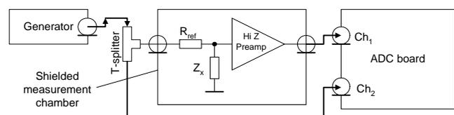
Fig. 1. Measurement setup
