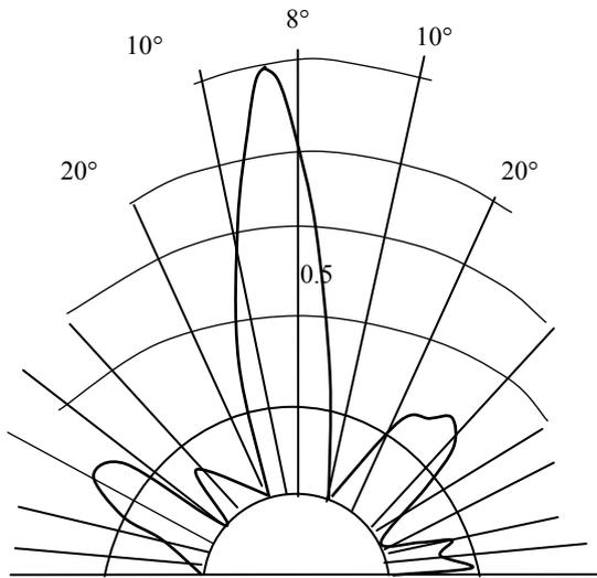
Fig.5. Directivity pattern of acoustic antenna (Fig. 4)
