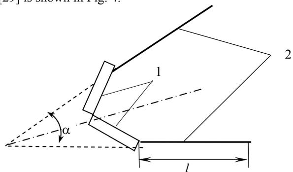
Fig.4. Cross section of unidirectional acoustic antenna: 1 – rectangular bimorph piezotransducers; 2 – reflectors of acoustic waves
