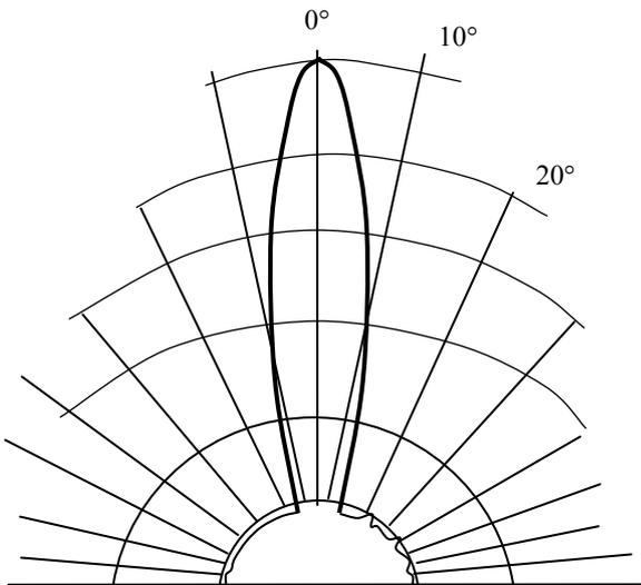
Fig.10. Directivity pattern of acoustic antenna (Fig. 9)
