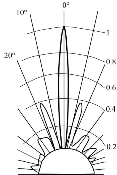
Fig.7. Directivity pattern of acoustic antenna (Fig. 6)
