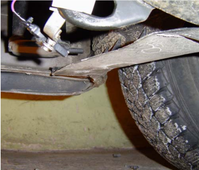
Fig. 3. Transducer placement under the car
