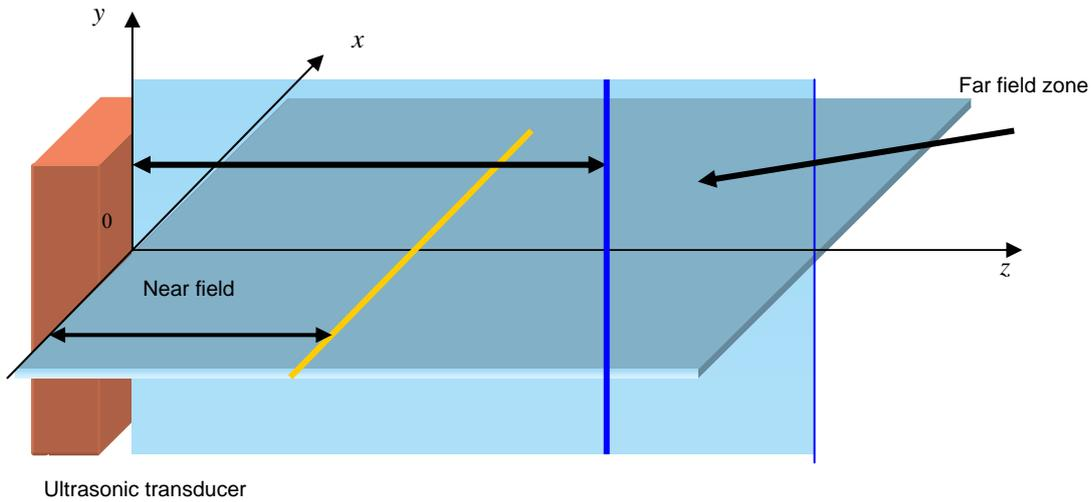
Fig. 4. Ultrasonic field of rectangular transducer in  $x0z$  and  $y0z$  planes
