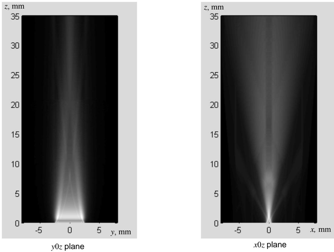
Fig. 6. Ultrasonic field of 5MHz transducer with dimensions 1x5 mm
