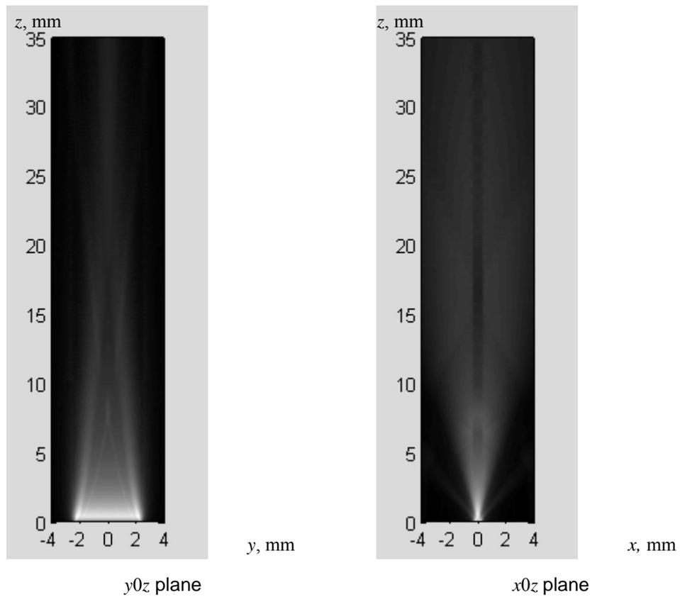
Fig. 10. Ultrasonic fields in a transmission mode of 10 MHz transducer (0.7×5 mm)
