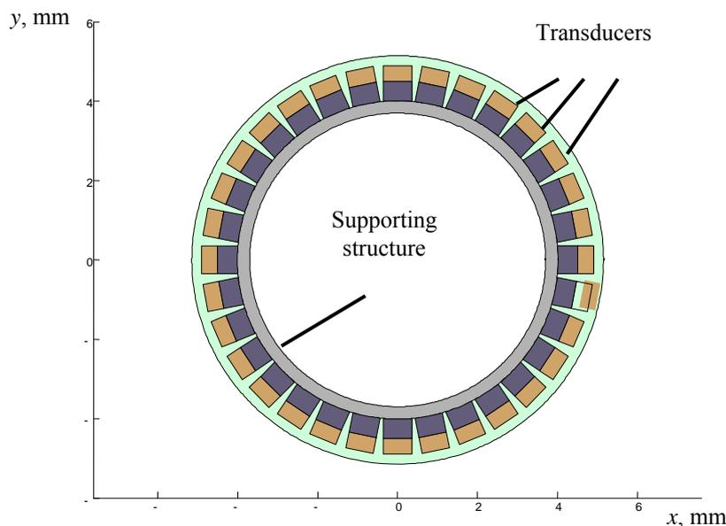
Fig.1 Ultrasonic array consisting of 32 separate transducers
