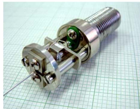
Fig. 15. Stainless steel wave guide with the bonded piezoelement after the \gamma -irradiation
