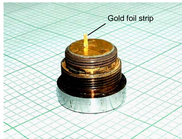
Fig. 11. Thick protector with the diffusion bonded piezoelement and gold foil strip
