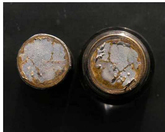
Fig. 13. Delaminations in bismuth titanate piezomaterial when the pressure or/and the temperature were too large for this piezoelectric material. In a tensile strength
