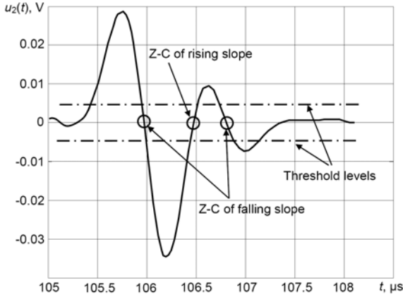
Fig.1. The zero crossing detection and determination of the singular zero crossing time moments according to rising or falling slopes of the signal transmitted through the human head u_2(t)
