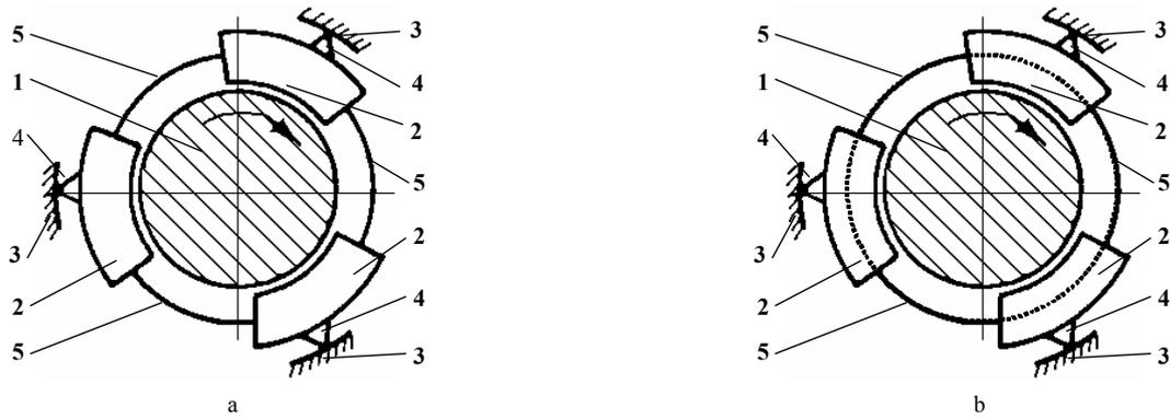
Fig. 2. Adaptive hydrodynamic bearings: a – elastic shoulders that are connected segments: 1 - rotor, 2 – segments 3 - spindle head 4 - adaptive thrust; 5 - elastic shoulders that are connected segments; b – with elastic ring that is moved easily and is connected segments: 1 - rotor, 2 – segments 3 - spindle head 4 - adaptive thrust, 5 - elastic ring
