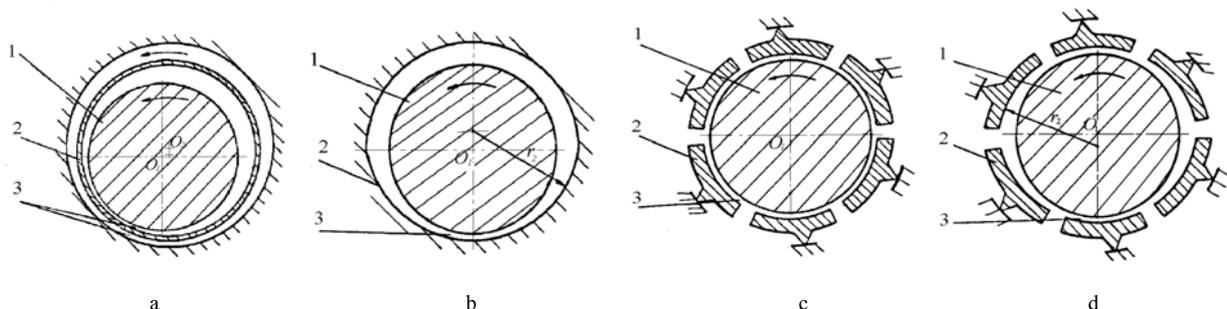
Fig. 1. Bearings : a – self-adjustment including floating ring bearings, b – elliptical bearings, c - tilting-pad journal bearings, d - elliptical tilting pad journal bearings; 1 - rotor, 2 - floating spacer or segment, 3 - carrying lubricating layer
