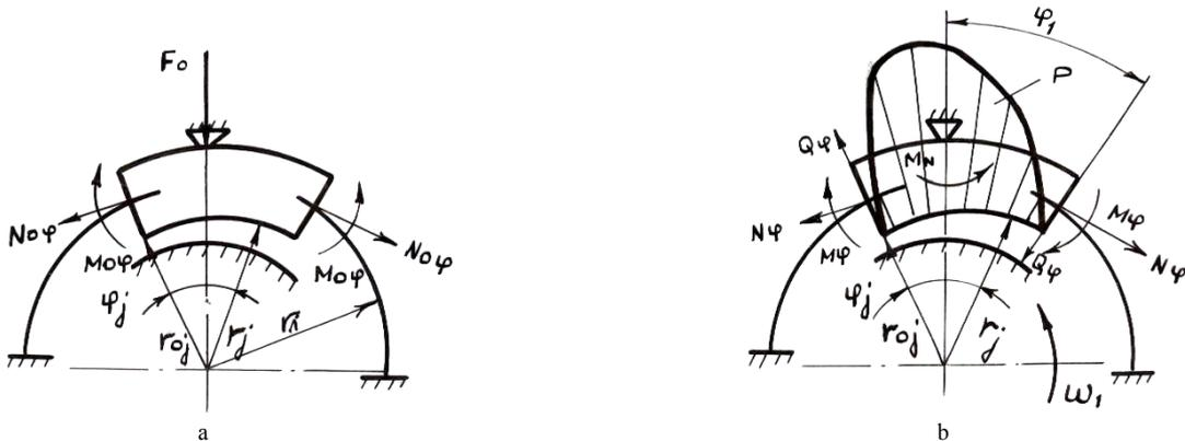
Fig. 3. Powers that are operated on segments of bearing: a – being preconceived weighting, b – being hydrodynamic pressure
