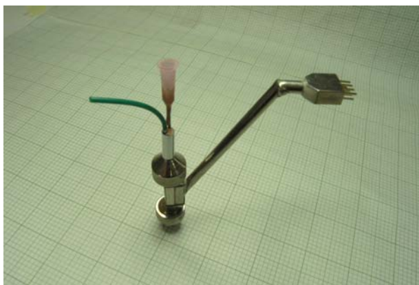
Fig. 3. Photo of the four-channel 0.7 ml volume chamber, immersed in a water bath during the experiment
