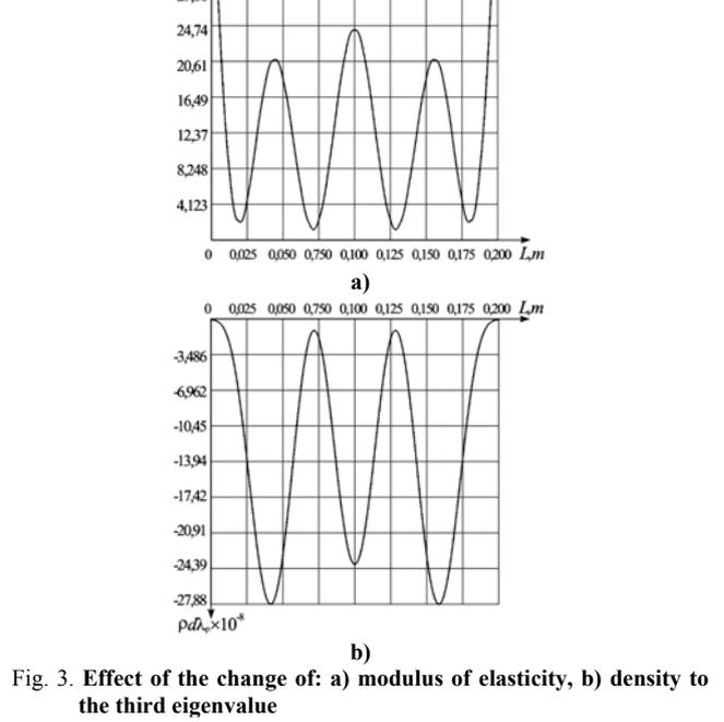
Fig. 3. Effect of the change of: a) modulus of elasticity, b) density to the third eigenvalue
