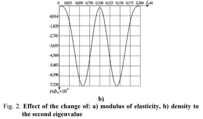
Fig. 2. Effect of the change of: a) modulus of elasticity, b) density to the second eigenvalue
