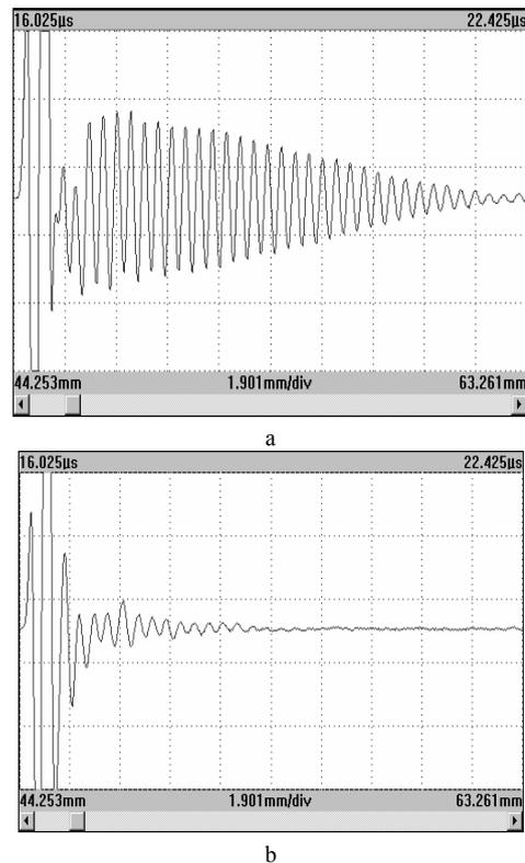
Fig. 2. First ultrasonic pulse reflected form the external surface of a steel pipe displaying the ringing effect for the gluing absence (a) and the pulse for the proper gluing (b); broadband, 5 MHz probe was used
