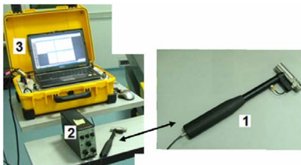
Fig. 2. Equipment used for impact excitation ("Brüel & Kjær"): 1) the impact hammer 8202 with the force transducer 8200, 2) the amplifier 2626, 3) the portable measurement results processing station „Machine Diagnostics Toolbox Type 9727“ ("Brüel & Kjær")
