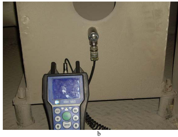
Fig. 5. Vibration velocity spectrum of the third blower frame at 8A measurement point (a) and vibration measurement general view at point 5A (b)
