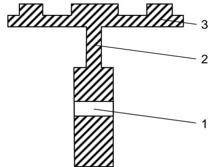
Fig. 10. Schematic diagram of composite transducer with transformation of vibrations: 1 – magnetostrictive transducer; 2 – concentrator of acoustic waves; 3 – circular radiating element
