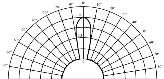
Fig. 9. Radiation pattern of acoustic antenna (Fig. 8)
