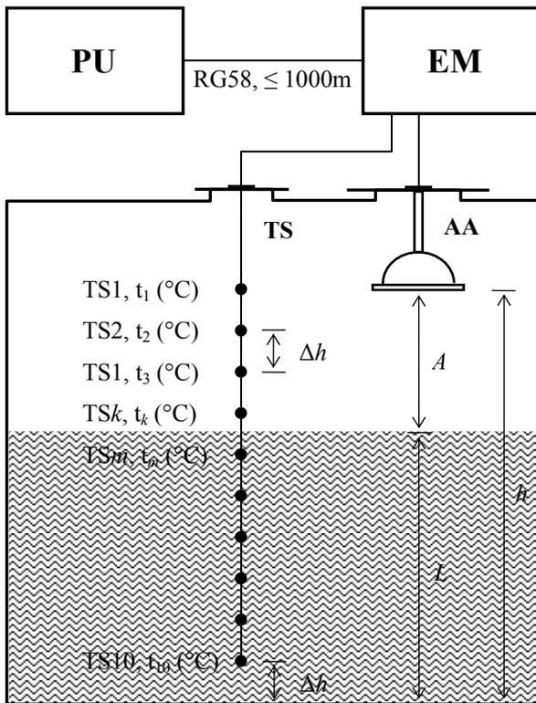
Fig. 12. Schematic diagram of the ultrasonic level measurement system with environmental temperature evaluation: TS – array of temperature sensors; AA – unidirectional acoustic antenna
