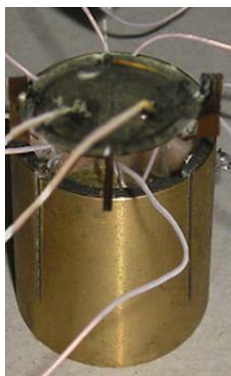
Fig.5. Experimental sample of bimorph of the tubular piezoceramic scanner
