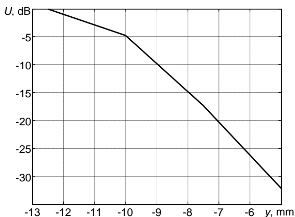
Fig.18. Dependence of the amplitude of the reflected signals from the distance of the defect from the top surface of the rail (log scale)
