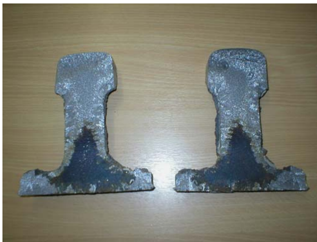
Fig.11. Photo of the rail with the shrinkage defect
