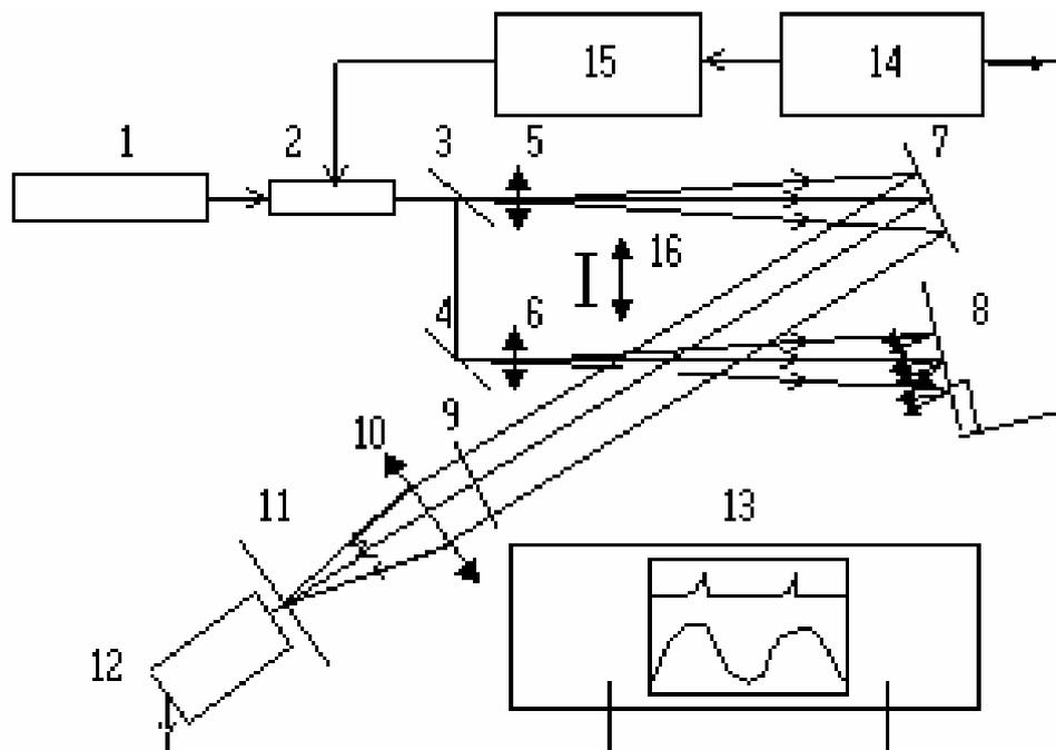
Fig 5. The experimental equipment diagram: 1-laser, 2-shutter, 3,4,7-mirrors, 5,6,10-lenses, 8-modulator,
