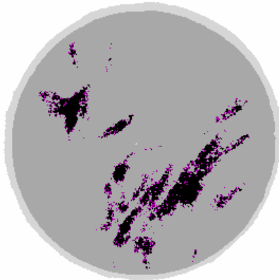
Fig. 8. Zoomed area of X-radiograph, presenting examined hole.
