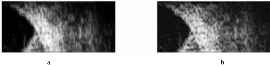
Fig. 6. Original a) and deconvolved b) with modelled PSF fragment of the image
