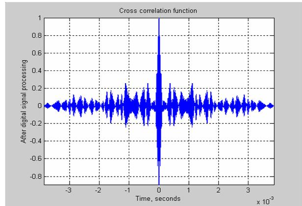
Fig.13. Normalized cross correlation function between the mixture of 60 PN- signals and the reference signal after digital signal processing
