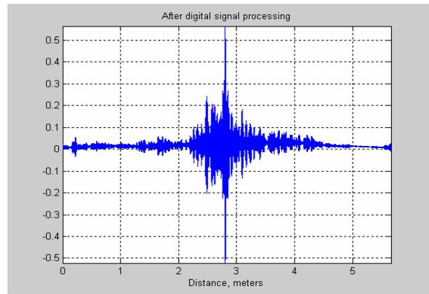
Fig.19. Normalized cross correlation function between the mixture of PN- signals and the reference signal after digital signal processing
