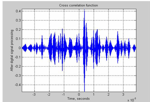
Fig.15. Normalized cross correlation function between the mixture of 10 PN- signals and the reference signal after digital signal processing
