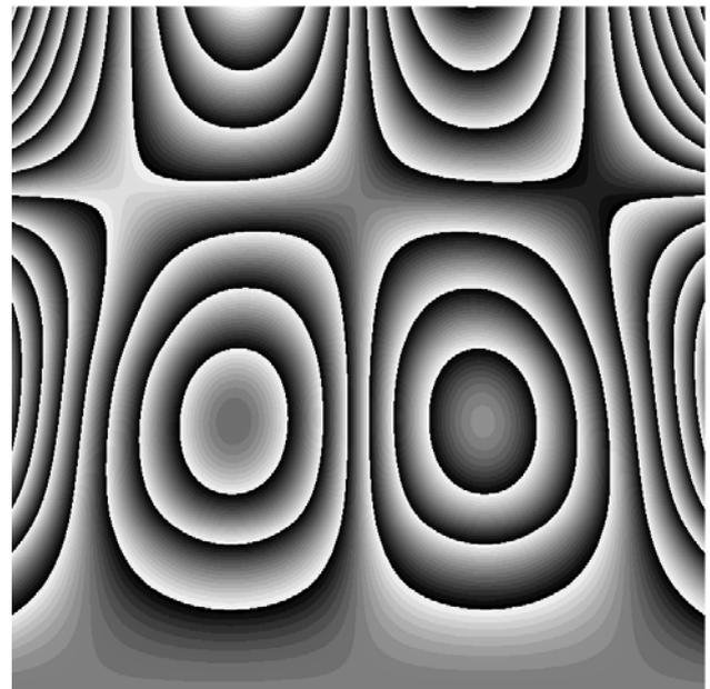
Fig. 6. The tenth eigenmode of the deflection of the plate
