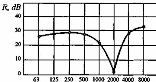
Fig. 2.1. Sound insulation frequency dependence of a housing
