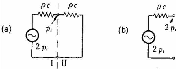
Fig. 2. Analogous circuit: (a) Open air and (b) Rigid wall
