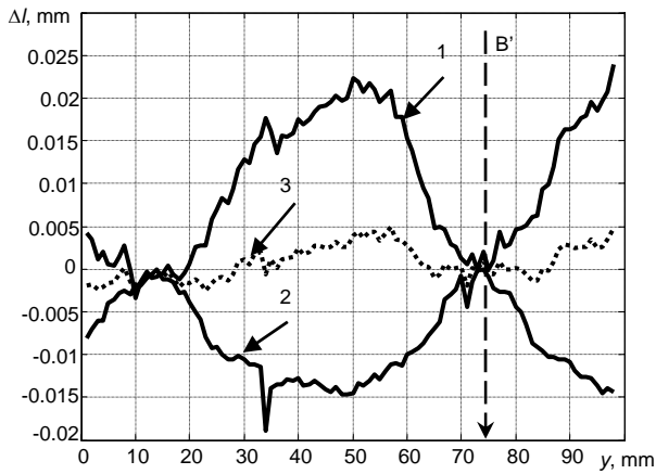
Fig. 6. Thickness measurement with different techniques along the BB cross-section: 1-zero-crossing, 2-cross-correlation, 3-average of the both techniques
