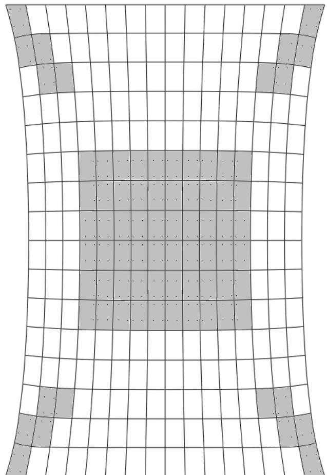
Fig.1. The statically distorted mesh with the points of numerical integration in the plastic region
