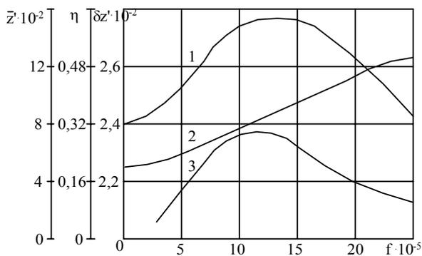
Fig.4. Dependencies of average velocity  $\bar{z}'$ , efficiency  $\eta$ , and non uniformity coefficient of motion  $\delta z'$  versus pressing force  $f$ : 1-  $\bar{z}'$ ; 2 -  $\eta$ ; 3 -  $\delta z'$ ,  $\psi_0 = 0.01$ ,  $h=0.05$ ,  $h_0=0.1$ ,  $f_0=0.05$ ,  $\omega/\omega_{\max} = 0.5$
