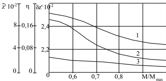
Fig.5. Dependencies of average velocity  $\bar{z}'$ , efficiency  $\eta$ , and non uniformity coefficient of motion  $\delta z'$  versus the output link mass  $M/M_{\max}$ : 1 -  $\bar{z}'$ ; 2 -  $\eta$ ; 3 -  $\delta z'$ ,  $\psi_0 = 0.01$ ,  $h=0.05$ ,  $h_0=0.1, f_0=0.05, f=8 \cdot 10^{-5}$ ,  $\omega/\omega_{\max} = 0.5$
