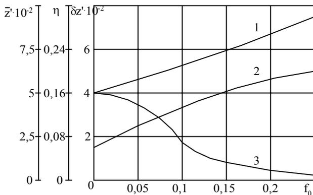
Fig 3 Dependencies of average velocity  $\bar{z}'$ , efficiency  $\eta$ , and non uniformity coefficient of motion  $\delta z'$  on dry friction coefficient  $f_0$ : 1 -  $\bar{z}'$ ; 2 -  $\eta$ ; 3 -  $\delta z'$ ,  $h=0.05$ ,  $h_0=0.01$ ,  $f=8 \cdot 10^{-5}$ ,  $\omega/\omega_{\max}=0.5$ ;  $\psi_0 = 0.01$
