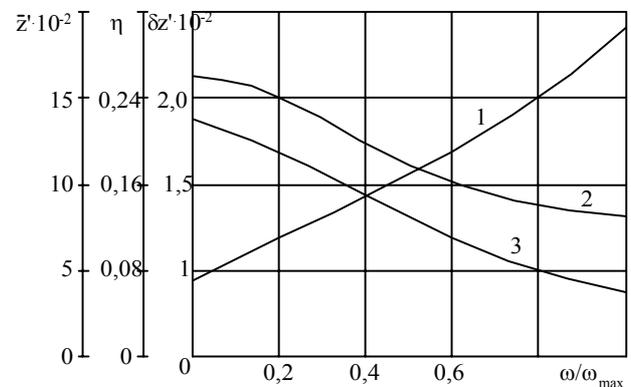
Fig.2. Dependencies of average velocity  $\bar{z}'$ , efficiency  $\eta$ , and non-uniformity coefficient of motion  $\delta$  versus frequency
