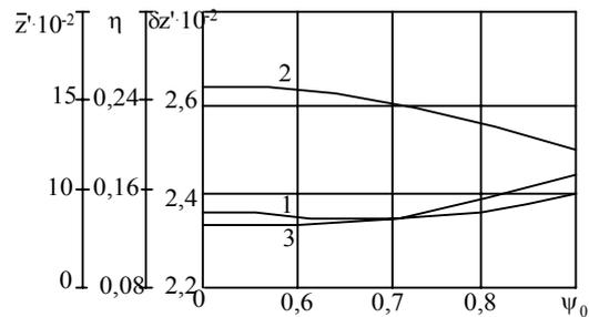
Fig.6. Dependencies of average velocity  $\bar{z}'$ , efficiency  $\eta$ , and non uniformity coefficient of motion  $\delta z'$  on phase shift  $\psi_0$ : 1 -  $\bar{z}'$ ; 2 -  $\eta$ ; 3 -  $\delta z'$ ,  $h=0.05$ ,  $h_0=0.1$ ,  $f_0=0.05$ ,  $f=8 \cdot 10^{-5}$ ,  $\omega/\omega_{\max} = 0.5$ .
